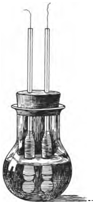
FIG. 2.—Iodine Concentration Cell, showing Stopped Electrodes.
